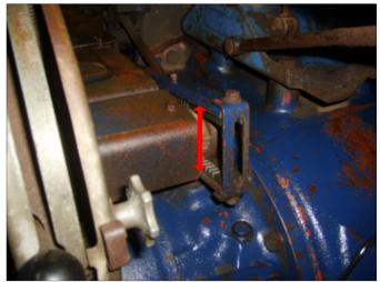
Remove the actuator pin. (If it's missing a new one MUST be obtained, it's vital to the correct operation of the hydraulics)
