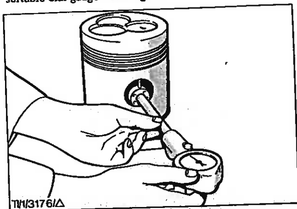
Fig. 34 - Measuring Piston Pin Bore
